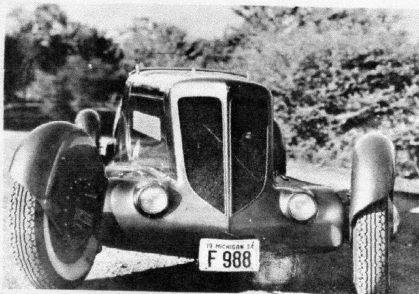
Long front end might have been made to simulate front-wheel drive, because at this time Edsel was involved in fwd Miller-Ford Indy assault. Low headlights, "shaved" look predate post-war hot rods.
